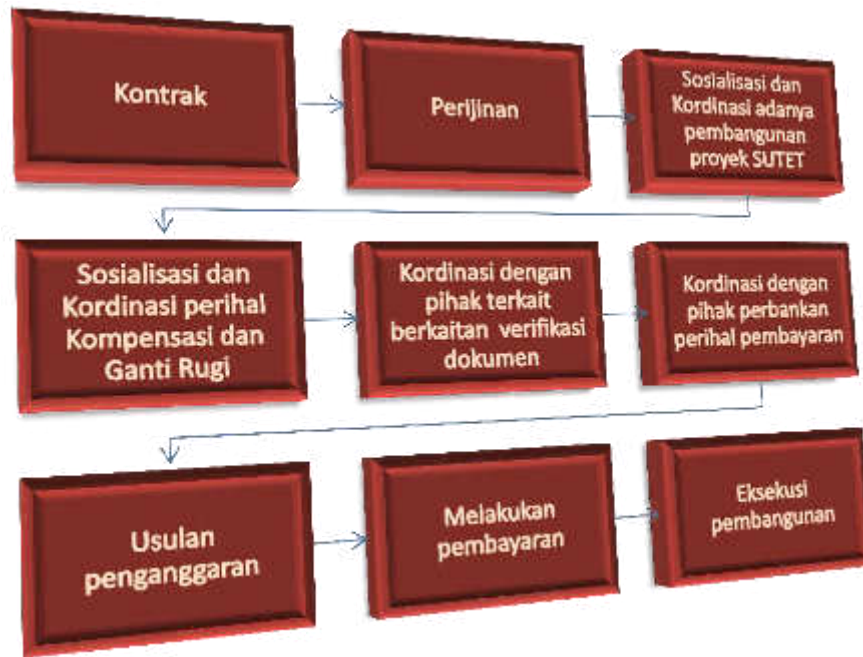
Figure 6 The process of land acquisition, land restriction, growing plant or building limitation located under RoW line of SUTT TL 150 kV Route Bengkayang – Ngabang – Tayan.
